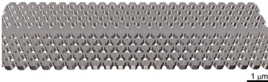
Figure: Optomechanical waveguide fabricated on silicon. This will be our basic geometry to study [3].
